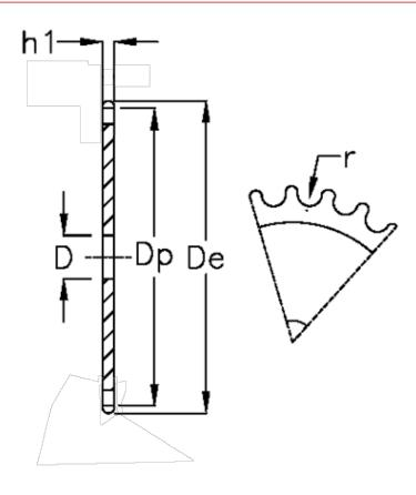
C = 2 D = 20 De = 232.9 Dp = 224.64 For chain size = 3/4 x 7/16 For chain type = 12 B-1 h1 = 11.1 Sumber of teeth = 37
